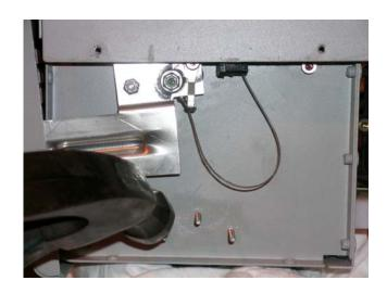
6. Mount the cable pulley C where the studs were with the 6-32 truss head screws that are in the cable pulley mounting plate.
