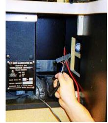
24-position connector of the existing harness into the BavSonic<sup>TM</sup> AW upgrade harness supplied in the kit. Plug the 3-position and 4-position connectors into their respective receptacles on the inside base audio board.
