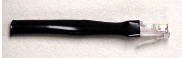
Test Plug used to test the intercom and Telephone Audio Interface
