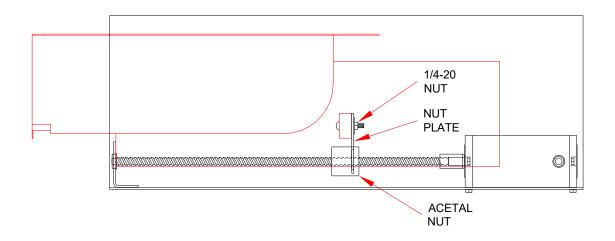
5. Push the Red Bin out far enough to gain access to the two nuts that secure the black Side Fillers, and then just loosen the two nuts that secure each of the side fillers. Once they are loose, lift the side fillers up and out of the drawer.
