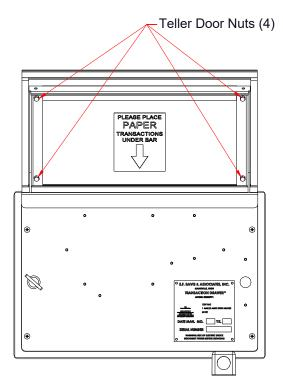
3. Remove the inside back cover, (5 screws for original, 4 screws on current).
