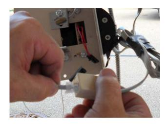
9. Connect the handset pigtail lead to the new hook switch wiring. Note that the connection is a four position connector with white and blue wires.
