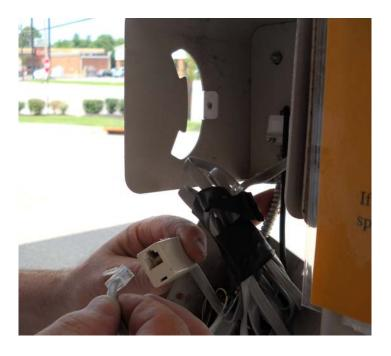
3. Remove screws to disassemble the hook switch assembly from the face plate.
