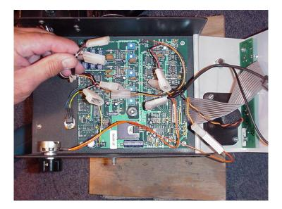
3. Unplug the Pre-amp from the old handset harness (3 position Molex connector plug) and plug into the 3-position Molex connector coming from the audio board (X5, X6, X7).
