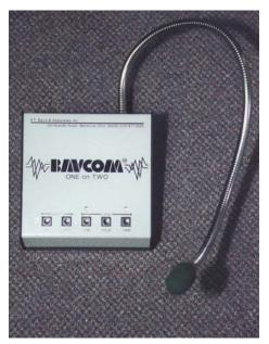
The BavCom **One on Two Audio** allows pharmacy personnel to speak with two remote positions. Normally this includes one internal station at the window and two external stations; one at the window and one at a second lane of service. As previously stated in the One on One section, full duplex operation is in place. Also, the inside console is the same 16ga steel construction with powder coat finish. However, the operator controls and logic are different with the **One on Two Audio**.
