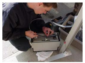
Mount the carrier to the drive tape. See page 9 and illustration on how to do this. Use the new short screws supplied on the small tape block. Use the new long screws that are supplied on the large tape block
