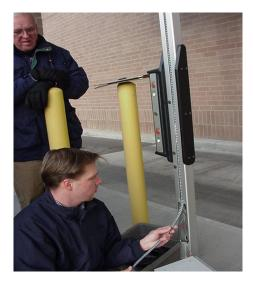
Insert the tape back into the customer vertical until the end of the tape engages the sprocket inside the machine. Note: While doing this if any obstructions or excess drag is felt, check and correct the problem.
