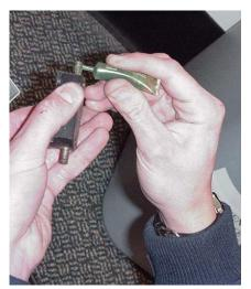
Lube the axles with the blue/green grease provided. Install the new brass wheels, (must be ordered separately), or reinstall the existing ones. Clean all excess grease off of the assembly so that it does not get on the tape or track. Make sure that the wheels turn freely.
