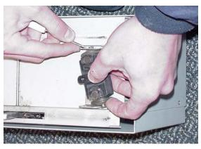
Remove the "E" clips that hold the large tape block and brass wheels in place.
